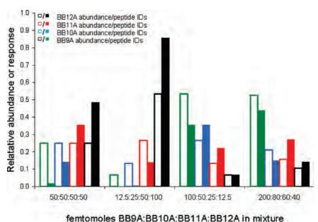
**Figure 5.** Peptide identifications from triplicate analyses of peptide library mixtures at differing relative abundances. Hollow bars indicate the solution-phase abundance of each library, whereas solid bars show the fraction of peptide identifications pertaining to particular libraries upon triplicate analysis of each mixture. Abundance ratios are given below each bar graph cluster in femtomoles of BB9A/BB10A/BB11A/BB12A, respectively.
