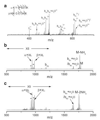
Figure 2. MS/MS spectrum of [73]KYIPGTK [79] crosslinked to [54]NKGITWK[60] (a) in ESI-Orbitrap (3+ precursor ion); (b) in MALDI-LTQ (1+ precursor) without WideBand activation, and (c) with WideBand activation (peaks labeled by \* correspond to the loss of ammonia from  $\alpha$ +XL or  $\beta$ +XL)
